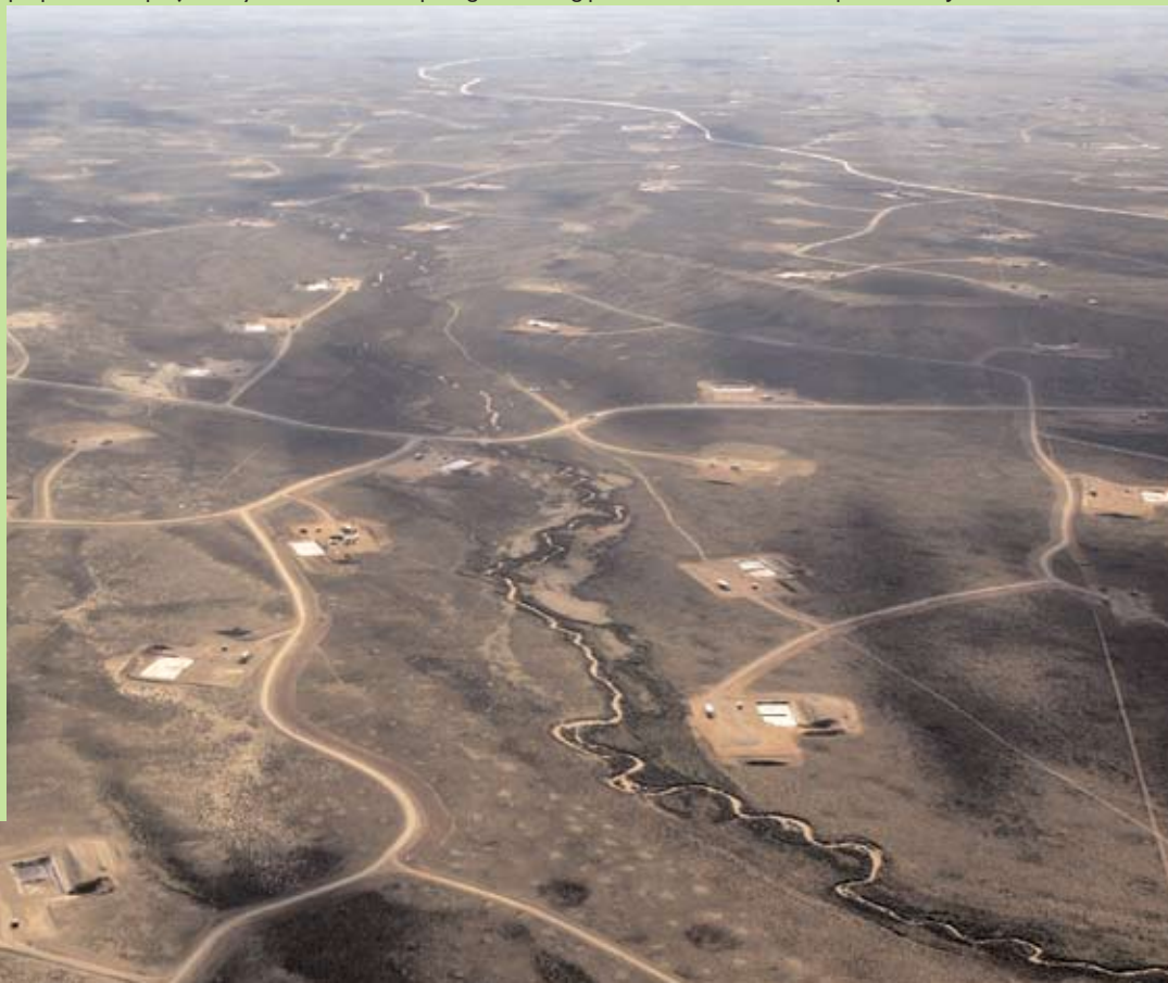
Below: Oil wells span the Upper Green River Valley's Jonah Field, where the wells are spaced 40 acres apart. A proposed infill project may add more wells, spacing the drilling pads as little as five acres apart. Photo: J. Selkowitz.
